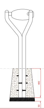
4 Fill hole with fast drying concrete to manufacturers specifications.
