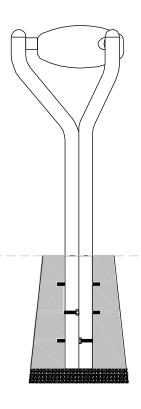
If Drum needs to be positioned lower a deeper hole can be excavated.
