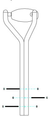
Excavate a holes with a 250mm diameter tapering down to 350mm diameter and 450mm depth
