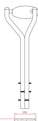
Compact base of hole with 50mm of aggregate. Lower ground Fix post attached to instrument into hole (check instrument straight and level before filling with concrete)
