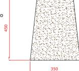
Foundations should not present a hazard. These foundations are recommended as a guide, for more information on foundation details for various surface see Part 7 of BS EN 1176.
