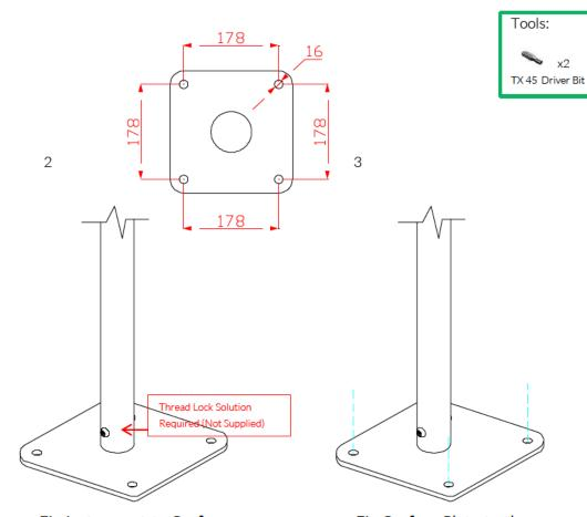
Fix instrument to Surface fix plate using M10 bolt and Barrel Nut and use **thread locking solution** to prevent fixings working loose.
