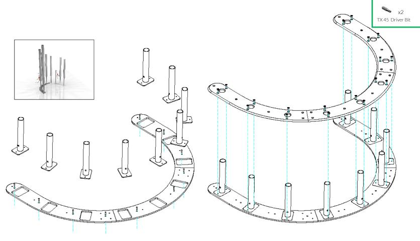
Mount this section of each base to the deck Deck Anchors Not provided using pre drilled holes
