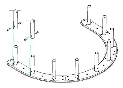
Lower Instrument over the stanchions and attach with fixings provided(see surface fix installation instructions)
