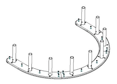
Join the upper and lower base sections with CSK M8x16mm Screws provided
